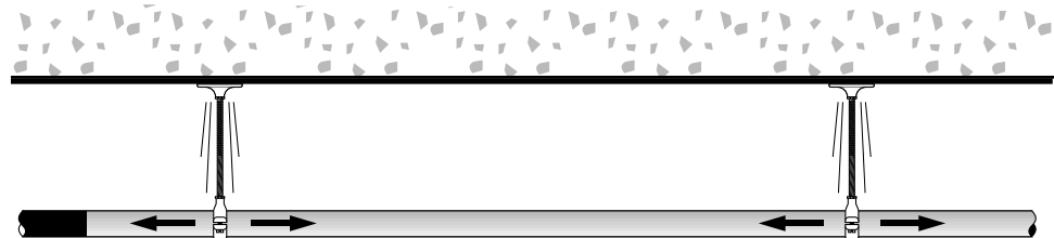
Fig. 3 When using extended pipe clamps the clamp should be loose enough to allow for expansion.
